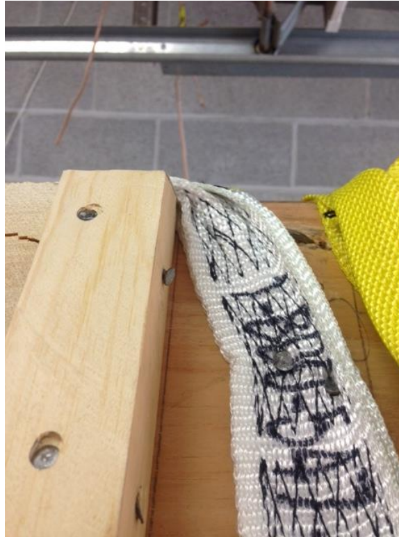
Photo 6: Polyester strap after testing (over ridge).
