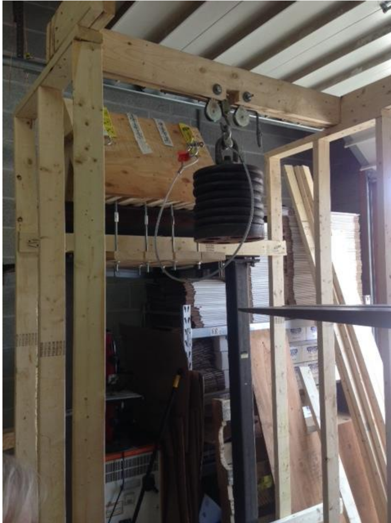
Photo 4: Temporary structure with quick release supporting 100kg (220lb) load.
