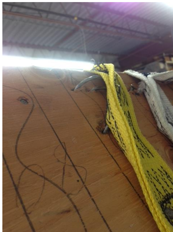
Photo 7: Nylon strap after testing (over ridge)
