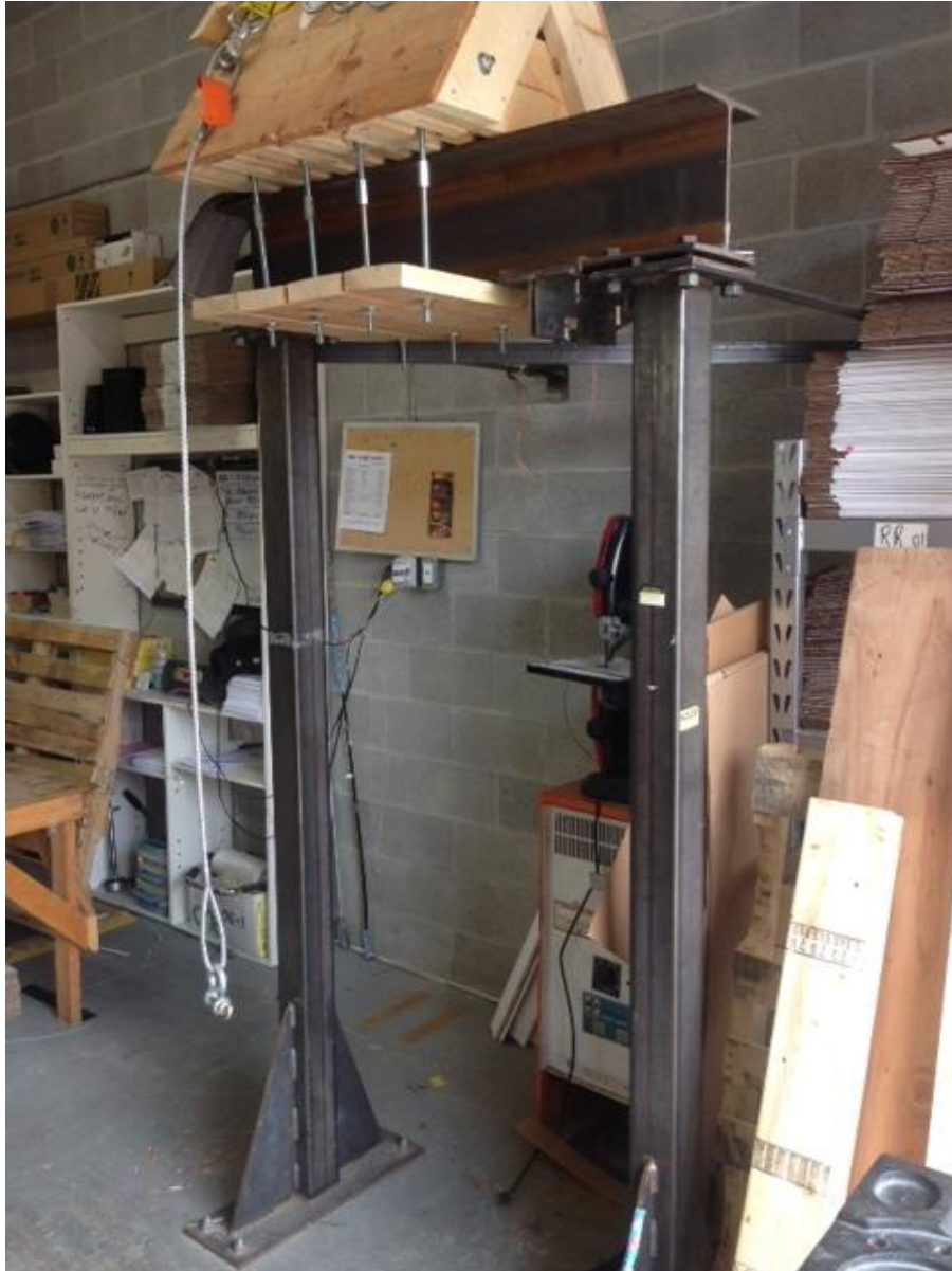
Photo 3: Structural Steel frame used for testing.
