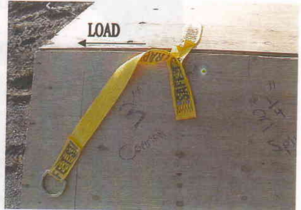
TEST 2 Load Parallel to nailed strap
